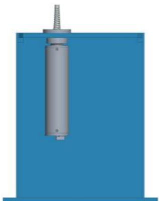
Figure 2-10: Installation in the water tank
