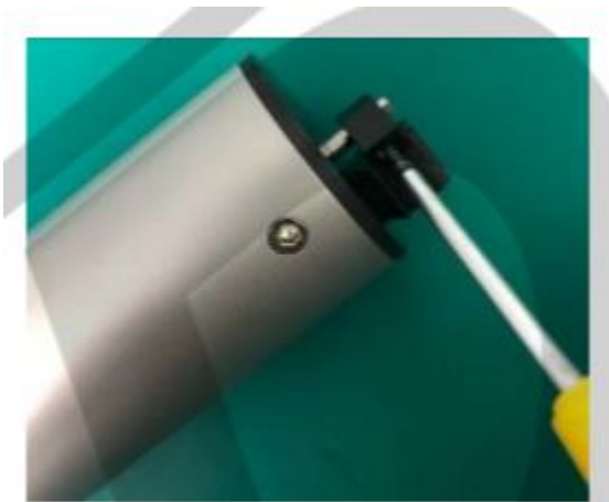
Figure 4-4: Removing the cleaning brush
