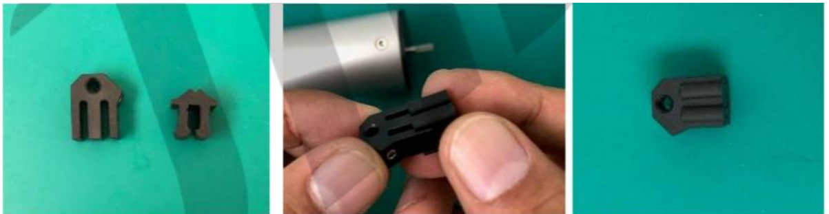
Figure 4-4: Removing the cleaning brush
